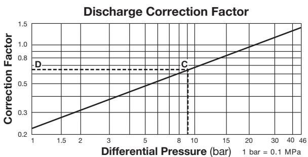
Differential pressure is the difference between the inlet and outlet pressure of the trap.
